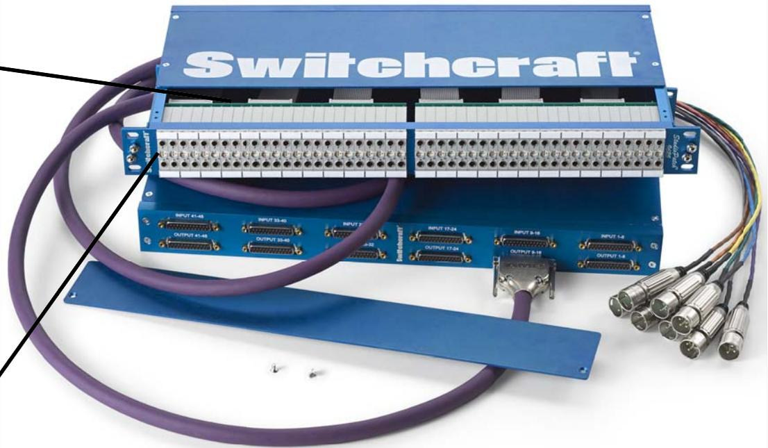
StudioPatch® Series audio patchbays utilize Switchcraft's EZ Norm technology, allowing signal flow to be changed from the front of the patchbay using a standard screwdriver. Now, every StudioPatch® Series patchbay comes with easy access programmable grounds, making it possible to custom configure the ground setting of each channel to either vertically strapped or isolated.
