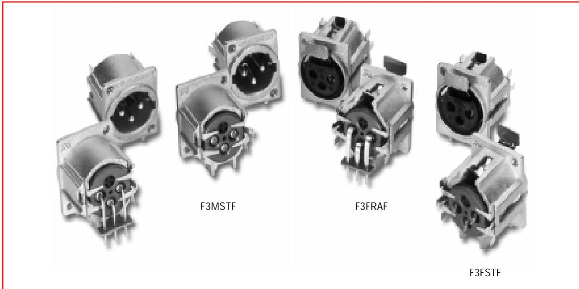
Switchcraft now offers the F Series. Available in male and female, the receptacles can be mounted from the rear of the panel. Features include an all metal housing with a ferrite disk for added EMI/RFI shielding. Both male and female connectors can be mounted vertical or horizontal to the PC board. All connectors have a PC-board retention feature to hold the connectors firmly to the PC board prior to soldering. See the chart below for part numbers.
