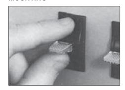
Grasp fingernail slots on opposite sides of escutcheon and snap out. Next, grasp lever and pull lever assembly free. Insert switch into panel hole.
