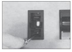
Turn two internal screws clockwise with screwdriver to securely mount switch to panel.
